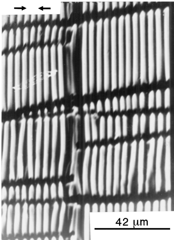
Figure 4 SEM micrograph of isoprene rubber, elongated without coating to 50%, coated with Pt film and released from grips.
